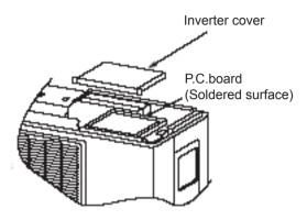
(2)As shown below, connect the discharge resistance (approx.100 $\Omega$ 20W) or plug of the sold ering iron to voltage between + - terminals of the electrolytic capacitor on PC Board for 30s, and then peformedischarging.
