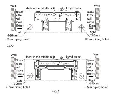
(2) Open a piping hole with the diameter of  $\Phi$ 55(70)mm on the selected outlet pipe position.In order to drain smoothly, slant the piping hole on the wall slightly downward to the outdoor side with the gradient of 5-10°.(As show in Fig.2)
