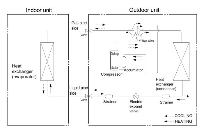
Connection pipe specification: Liquid pipe:1/4" (6mm) Gas pipe:1/2" (12mm) 18K Gas pipe:5/8" (16mm) 24K
