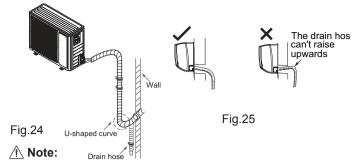
(1) The through-wall height of drain hose shouldnt be higher than the outlet pipe hole of indoor unit.(As show in Fig.25)
