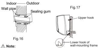
Do not bend the drain hose too excessively in order to prevent blockina.
