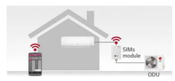
Monitor the status of your air conditioner and accurately diagnose problems by connecting it to a smartphone via a SIMs chip.
