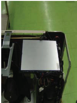
Remove Top Cover and Control Box Cover
